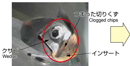
従来品 切くずづまりの状況 Conventional: Chips are clogged
