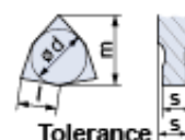
Tolerance s \pm 0.13 For l = 06, d \pm 0.05 m \pm 0.08 For l = 08, d \pm 0.08 m \pm 0.13
