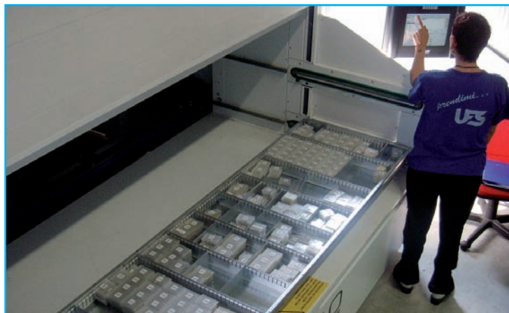
Automatic load system for final products
